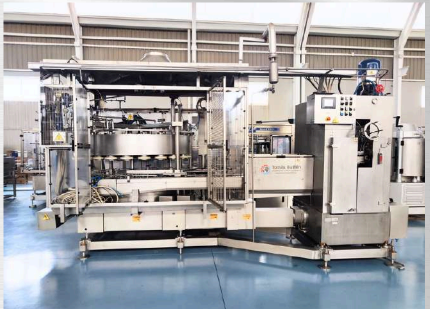
ANGELUS AUTOMATIC CAN SEAMER WITH ZILLI&BELLINI 36-VALVE VACUUM LIQUID FILLER
