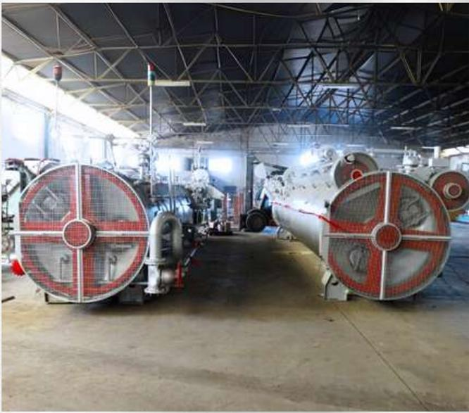
**AUTOCLAVE HORIZONTAL EN CONTINU FMC POUR BOÎTES**
