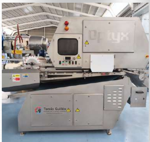
KEY OPTYX 3000 OPTICAL SORTER WITH DIGITAL CAMERA
