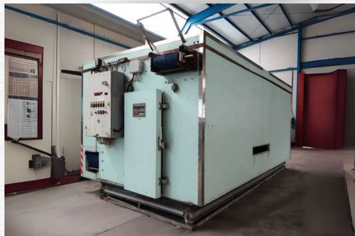
FRIGOSCANDIA SPIRAL IQF FREEZING TUNNEL
